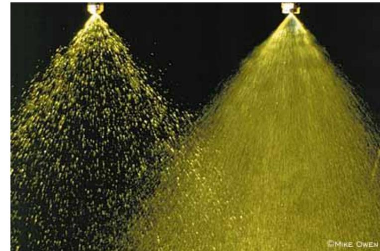
Figure II.1 Droplet size distribution of a Micron Ulva<sup>+</sup>, 7000 r.p.m., blank carrier oil, Odina EL and Shellsol T 1:1 (Bateman, in press).
